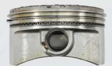
The piston and rings are virtually free of deposits and wear after 500 hours of severe-service testing in the Kawasaki\* FX 730 V engine.
