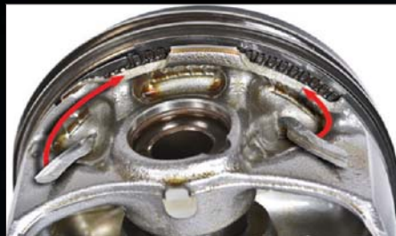
Example of piston damage due to an LSPI event observed during the testing of a competitor's motor oil. The red arrows indicate sections of the ring land that have broken away from the piston.
